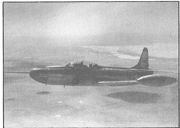
LeVier flying prototype model of the U.S. Air Force first allweather fighter (F-94A) made from Lockheed's first jet trainer TF-80 (T-33) which was made from the XP-80A #2.
